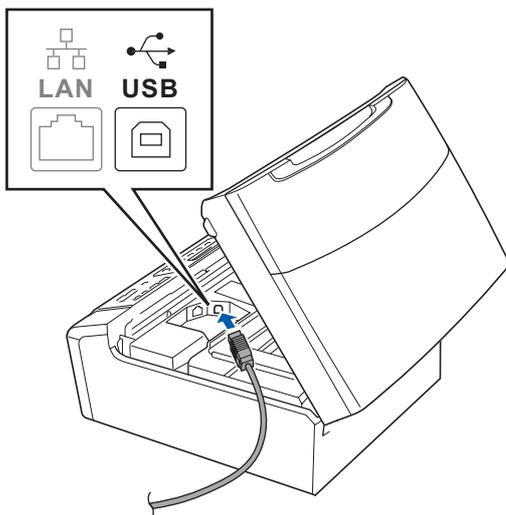
**c** Carefully route the USB cable through the trench and out the back of the machine as shown below and connect the cable to your computer.
