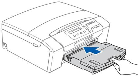
**i** While holding the paper tray in place, pull out the paper support **1** until it clicks, and then unfold the paper support flap **2**.
