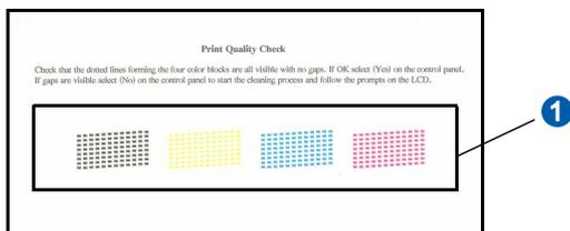
**c** If all lines are clear and visible, press ▲ (Yes) to finish the quality check and go to step **6**.
