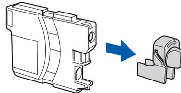
**f** Take care to match the color of the lever 1 with the cartridge color 2, as shown in the diagram below.
