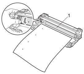
When you have found the mark on the drum that matches the print sample, wipe the surface of the OPC drum with a dry cotton swab until the dust or glue on the surface comes off.
