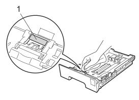
Wipe the two pick-up rollers (1) inside of the machine to remove dust.
