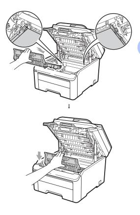
6 Slide each drum unit and toner cartridge assembly into the machine. Make sure that you match the toner cartridge color to the same color label on the machine. Repeat this for all the drum unit and toner cartridge assemblies.
