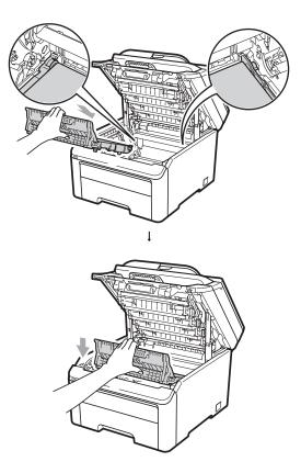
Slide each drum unit and toner cartridge assembly into the machine. Make sure that you match the toner cartridge color to the same color label on the machine. Repeat this for all the drum unit and toner cartridge assemblies.
