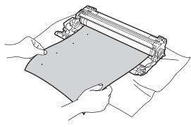
6 Turn the drum unit gear by hand while looking at the surface of the OPC drum (1).
