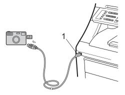
2 Turn on the camera. Make sure your camera is in PictBridge mode. When the machine has recognized the camera, the LCD shows the following message.
