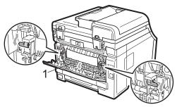
Using both hands, gently pull the jammed paper out of the fuser unit.
