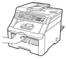
4 Using both hands, slide the manual feed slot paper guides to the width of the paper that you are going to use.
