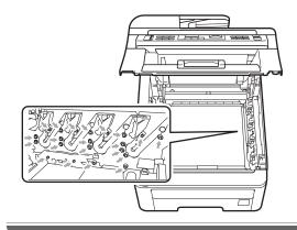
Clean the primary corona wire inside the drum unit by gently sliding the green tab from left to right and right to left several times.
