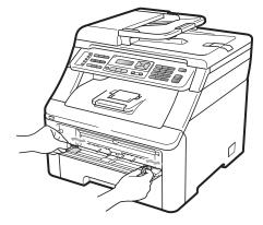
3 Using both hands, put one blank sheet of paper in the manual feed slot until the front edge of the paper touches the paper feed roller. Wait until the machine automatically feeds the paper. When you feel the machine pull in the paper, let go.
