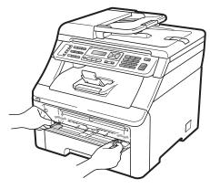
Using both hands, put one piece of paper in the manual feed slot with the print side face up until the front edge of the paper touches the paper feed roller. Wait until the machine automatically feeds the paper. When you feel the machine pull in the paper, let go.
