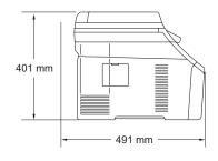
WeightWithout Drum/Toner Unit:20.1 kgNoise levelSound powerOperating (Printing):LWAd = 6.5 Bell (A)Standby:LWAd = 4.8 Bell (A)Sound pressureOperating (Printing):Operating (Printing):LPAm = 53 dB (A)Standby:LPAm = 30 dB (A)
