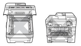
To prevent injuries, be careful not to put your hands on the edge of the machine under the document cover, the scanner, or the top cover as shown in the illustrations.
