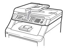
• You can still use the machine while the scanner is up. To close the scanner, push it down with both hands.
