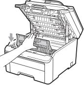
$\mathbf{10}$ Reinstall the original packing material into the machine.
