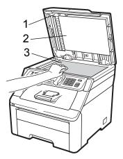
In the ADF unit, clean the white bar (1) and the scanner glass strip (2) underneath it with a soft lint-free cloth moistened with water.
