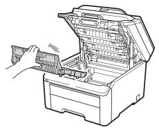
8 Remove the waste toner box from the machine, and then put it in a plastic bag and seal the bag completely.
