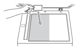
Even if a document is set on the ADF, the machine scans the data from the scanner glass.
