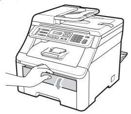
4 Using both hands, slide the manual feed slot paper guides to the width of the paper that you are going to use.
