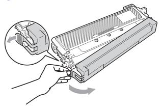
8 Put the new toner cartridge firmly into the drum unit until you hear it lock into place.
