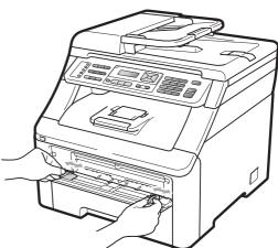
3 Using both hands, put one blank sheet of paper in the manual feed slot until the front edge of the paper touches the paper feed roller. Wait until the machine automatically feeds the paper. When you feel the machine pull in the paper, let go.
