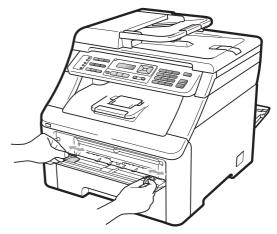
Using both hands, put one sheet of paper or one envelope in the manual feed slot until the front edge of the paper or envelope touches the paper feed roller. When you feel the machine pull in the paper, let go.
