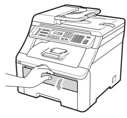
Using both hands, slide the manual feed slot paper guides to the width of the paper that you are going to use.
