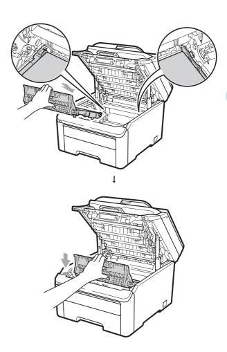
Slide each drum unit and toner cartridge assembly into the machine. Make sure that you match the toner cartridge colour to the same colour label on the machine. Repeat this for all the drum unit and toner cartridge assemblies.
