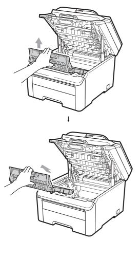
8 Remove the waste toner box from the machine, and then put it in a plastic bag and seal the bag completely.
