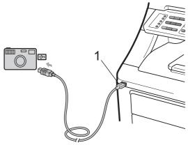
Turn on the camera. Make sure your camera is in PictBridge mode. When the machine has recognized the camera, the LCD shows the following message depending on which mode the machine is in:
