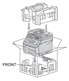
Put the power cord, and the three remaining drum unit and toner cartridge assemblies into the Styrofoam pieces as shown in the illustration.
