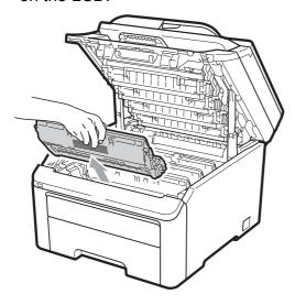
4 Push down the green-labelled lock lever (1) and take the toner cartridge out of the drum unit.
