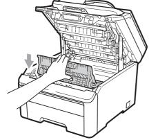
Slide each drum unit and toner cartridge assembly into the machine. Make sure that you match the toner cartridge color to the same color label on the machine. Repeat this for all the drum unit and toner cartridge assemblies.
