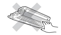
4 Hold the green handle of the belt unit and lift the belt unit up, then pull it out.
