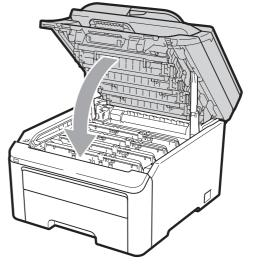
1 Plug the machine's power cord back into the AC power outlet first, and reconnect all cables and the telephone line cord. Turn on the machine's power switch.
