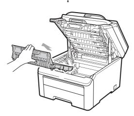
Remove the waste toner box from the machine, and then put it in a plastic bag and seal the bag completely.
