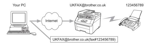
You can also send E-mail from your computer and have it relayed to a conventional fax machine. The method of entering the phone number of the conventional fax machine that will receive the relayed E-mail will vary depending on the mail application you are using. The following are some examples of different mail applications:
