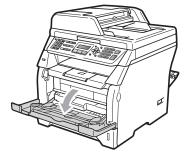
4 Pull out the MP tray support (1) and unfold the flap (2).
