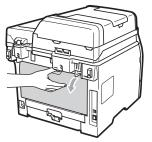
Pull the tabs at the left and right hand sides toward you to open the fuser cover (1).
