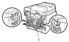
6 Pull the jammed paper out of the fuser unit.
