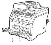
5 While pressing the paper side guide release lever, slide the paper guides to fit the width of the paper that you are going to use.
