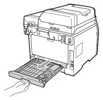
2 Pull the jammed paper out of the machine or the duplex tray.
