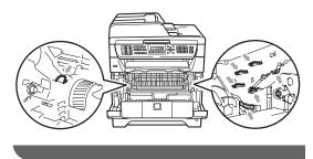
Clean the corona wire inside the drum unit by gently sliding the blue tab from right to left and left to right several times.
