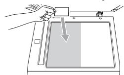
Even if a document is set on the ADF, the machine scans the data from the scanner glass.
