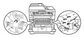
Push down the blue lock lever and take the toner cartridge out of the drum unit.
