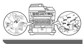
3 Push down the blue lock lever and take the toner cartridge out of the drum unit.
