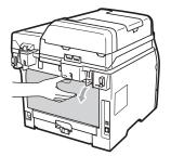
5 Pull the tabs at the left and right hand sides toward you to open the fuser cover (1).
