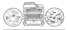
6 Put the drum unit and toner cartridge assembly back in the machine.
