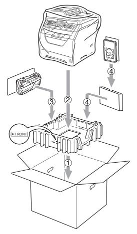
9 Take the two styrofoam pieces and match the front of the machine to the "FRONT" mark on one of the styrofoam pieces, and the back of the machine to the "REAR" mark on the other styrofoam piece (5). Coil the cables and place them and the Quick Setup Guide in the spaces provided as shown below (6).
