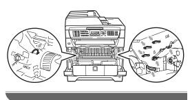
Bush down the blue lock lever and take the used toner cartridge out of the drum unit.
