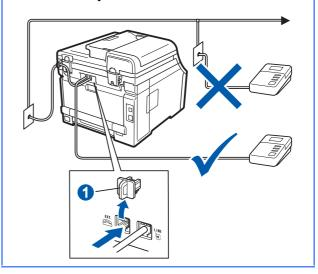
Set the receive mode to External TAD if you have an external answering machine. See Choose a Receive Mode on page 8. For additional details, see Connecting an external TAD in Chapter 7 of the User's Guide.
