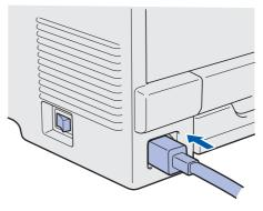
Plug the AC power cord into an AC outlet. Turn the power switch on.
