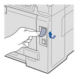
b Connect the USB cable to the USB connector on the machine marked with the symbol. Then connect the cable to your computer.
