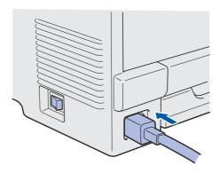
Plug the AC power cord into an AC outlet. Turn the power switch on.
