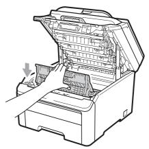
9 Reinstall the original packing material into the machine.
