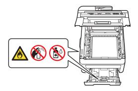
DO NOT use a vacuum cleaner to clean up scattered toner. Doing this might cause the toner dust to ignite inside the vacuum cleaner, potentially starting a fire. Please carefully clean the toner dust with a dry, lint-free soft cloth and dispose of it according to local regulations.
