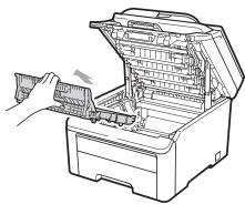
Remove the waste toner box from the machine, and then put it in a plastic bag and seal the bag completely.
