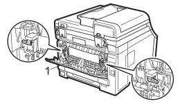
4 Using both hands, gently pull the jammed paper out of the fuser unit.
