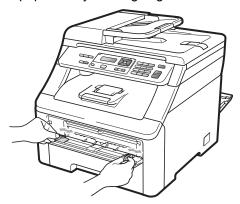
5 Using both hands, put one sheet of paper or one envelope in the manual feed slot until the front edge of the paper or envelope touches the paper feed roller. When you feel the machine pull in the paper, let go.
