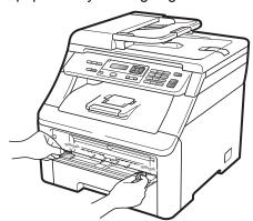
Using both hands, put one blank sheet of paper in the manual feed slot until the front edge of the paper touches the paper feed roller. Wait until the machine automatically feeds the paper. When you feel the machine pull in the paper, let go.
