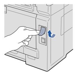
Connect the USB cable to the USB connector on the machine marked with the 🚭 symbol. Then connect the cable to your computer.
