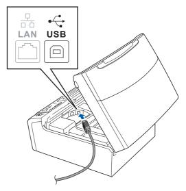
Carefully guide the USB cable through the trench as shown below, following the trench around and toward the back of the machine. Then connect the cable to your Macintosh.
