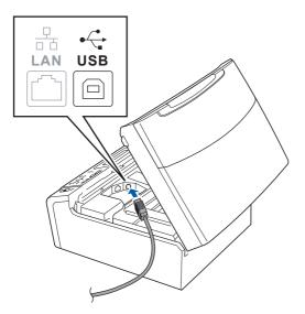
Carefully guide the USB cable through the trench as shown below, following the trench around and toward the back of the machine. Then connect the cable to your computer.
