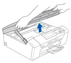
Connect the network cable to the LAN socket marked with a symbol. You will find the LAN socket inside the machine on the left as shown below.
