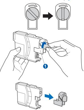
Take care to match the colour of the lever **1** with the cartridge colour **2**, as shown in the diagram below.
