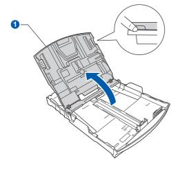
C With both hands, gently press and slide the paper side guides 1 and then the paper length guide 2 to fit the paper size you are loading in the tray.
