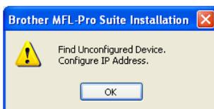
Click **OK** and then click **Configure IP Address**. Enter an IP address for your machine that is suitable for your network by following the on-screen instructions.
