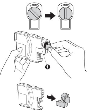
Take care to match the colour of the lever **()** with the cartridge colour **(2)**, as shown in the diagram below.
