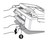
C Remove the plastic bag containing the ink cartridges from on top of the paper tray.
