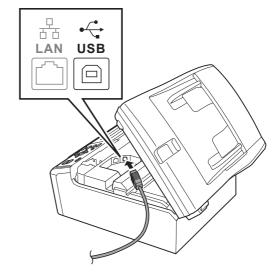
C Carefully guide the USB cable through the trench as shown below, following the trench around and toward the back of the machine. Then connect the cable to your computer.
