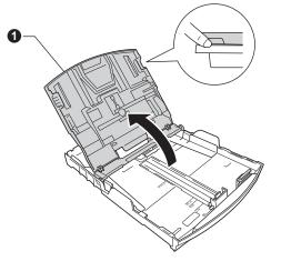
C With both hands, gently press and slide the paper side guides ● and then the paper length guide ❷ to fit the paper size.
