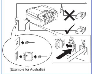
Set the receive mode to External TAD if you have an external answering machine. See Choose a Receive Mode on page 8. For additional details, see Connecting an external TAD (telephone answering device) in chapter 6 in the Basic User's Guide.
