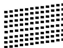
If you can see missing short lines, press **2 (No)** on the dial pad and follow the steps on the LCD.
