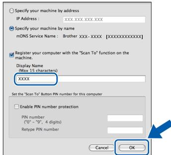
The name you enter will appear on the machine's LCD when you press the **SCAN** key and choose a scan option. (For more information, see Network Scanning (For models with built-in network support) in the Software User's Guide on the documentation CD-ROM.)
