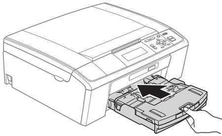
**i** While holding the paper tray in place, pull out the paper support ① until it clicks, and then unfold the paper support flap ②.
