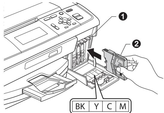
**g** Install each ink cartridge in the direction of the arrow on the label.
