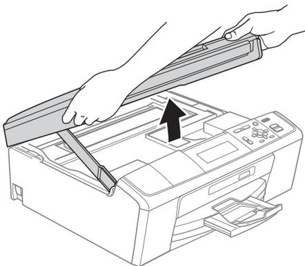
**b** Connect the USB cable to the USB socket marked with a
