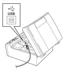
Carefully guide the USB cable through the trench as shown below, following the trench around and toward the back of the machine. Then connect the cable to your computer.
