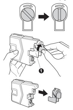
Take care to match the colour of the lever with the cartridge colour 2, as shown in the diagram below.
