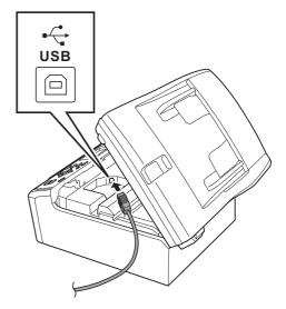
Carefully guide the USB cable through the trench as shown below, following the trench around and toward the back of the machine. Then connect the cable to your Macintosh.
