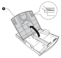
With both hands, gently press and slide the paper side guides • and then the paper length guide • to fit the paper size.
