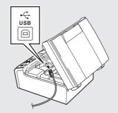
**C.** Carefully route the USB cable through the trench and out the back of the machine. Connect the cable to your Macintosh.
