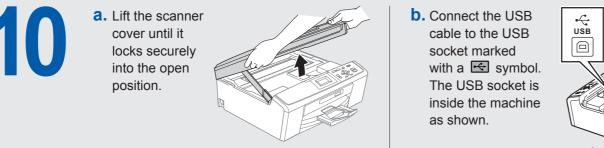
cable to the USB socket marked with a 🔄 symbol. The USB socket is inside the machine as shown.
