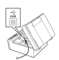
**C.** Carefully route the USB cable through the trench and out the back of the machine. Connect the cable to your computer.
