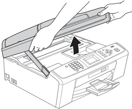
**b** Connect the USB cable to the USB socket marked with a
