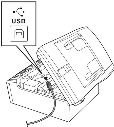
**c** Carefully guide the USB cable through the trench as shown below, following the trench around and toward the back of the machine. Then connect the cable to your computer.
