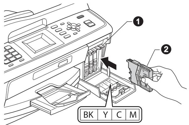
**g** Install each ink cartridge in the direction of the arrow on the label.
