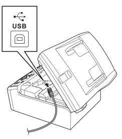
Carefully guide the USB cable through the trench as shown below, following the trench around and toward the back of the machine. Then connect the cable to your computer.
