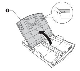
C With both hands, gently press and slide the paper side guides ● and then the paper length guide ❷ to fit the paper size.
