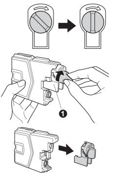
Take care to match the colour of the lever **①** with the cartridge colour **②**, as shown in the diagram below.
