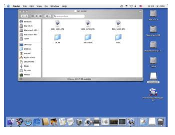
Quit all applications that are running stored data on the memory card or USB Flash memory drive and drag the **Removable Disk** icon into the **Trash** icon before you remove the memory card or USB Flash memory drive from the machine.
