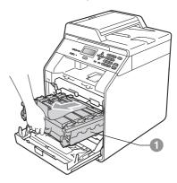
Gently pull the orange packing material towards the front of the machine to remove it.
