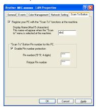
If you want to avoid receiving unwanted documents, enter a 4-digit PIN number in the **Pin number** and **Retype Pin number** field. To send data to a PC protected by a PIN number, the LCD prompts you to enter the PIN number before the document can be scanned and sent to the PC. (See *Using the Scan key on your network* on page 220.)
