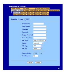
You can set Passive Mode to OFF or ON depending on your FTP server and network firewall configuration. By default this setting is ON. You can also change the port number used to access the FTP server. The default for this setting is port 21. In most cases these two settings can remain as default.
