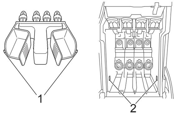
If you are not able to find the green protective part, DO NOT remove the ink cartridges before shipping. It is essential that the machine be shipped with either the green protective part or the ink cartridges in position. Shipping without them will cause damage to your machine and may void your warranty.
