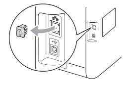
Connect the network interface cable to the LAN connector and then connect it to a free port on your hub.
