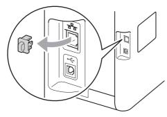
Connect the network interface cable to the LAN connector and then connect it to a free port on your hub.
