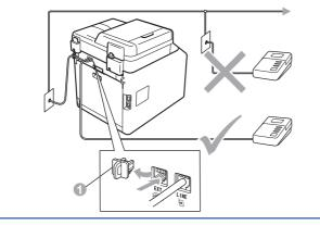
Set the receive mode to External TAD if you have an external answering machine. See Choose a Receive Mode on page 7. For additional details, see Connecting an external TAD in the Basic User's Guide.
