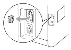
C Connect the network interface cable to the LAN connector and then connect it to a free port on your hub.
