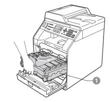
Gently pull the orange packing material towards the front of the machine to remove it.
