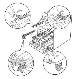
g Push the drum unit firmly back into the machine.
