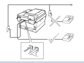
Set the receive mode to External TAD if you have an external answering machine. See Choose a Receive Mode on page 5. For additional details, see Connecting an external TAD in the Basic User's Guide.
