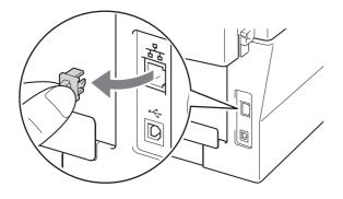
Connect the network interface cable to the LAN connector and then connect it to a free port on your hub.
