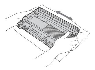
Put the drum unit and toner cartridge assembly back in the machine.
