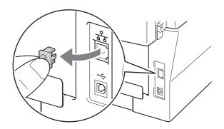
C Connect the network interface cable to the LAN connector and then connect it to a free port on your hub.
