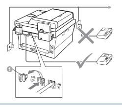
Set the receive mode to External TAD if you have an external answering machine. See Choose the correct Receive Mode on page 8. For additional details, see Connecting an external TAD (telephone answering device) in the Basic User's Guide.
