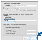
The name you enter will appear on the machine's LCD when you press the SCAN key and choose a scan option. (For more information, see Network Scanning in the Software User's Guide.)
