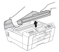
Connect the USB cable to the USB socket marked with a 😪 symbol. You will find the USB socket inside the machine on the right as shown below.
