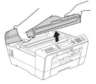
Store the orange protective part in the holder inside the machine as shown. Make sure that the two projections on the bottom of the orange protective part fit in the two slots in the holder.
