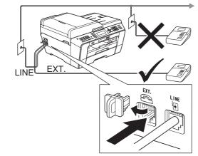
Set the receive mode to External TAD if you have an external answering machine. See Choose a Receive Mode on page 8. For additional details, see Connecting an external TAD (telephone answering device) in chapter 6 of the Basic User's Guide.
