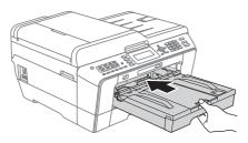
While holding the paper tray in place, pull out the paper support **①** until it clicks, and then unfold the paper support flap **②**.
