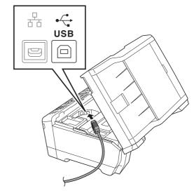
C Carefully guide the USB cable into the cable channel and out the back of the machine. Connect the cable to your computer.
