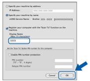
The name you enter will appear on the machine's LCD when you press the **SCAN** key and choose a scan option. (For more information, see Network Scanning in the Software User's Guide.)
