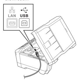
Carefully guide the USB cable into the cable channel and out the back of the machine.
