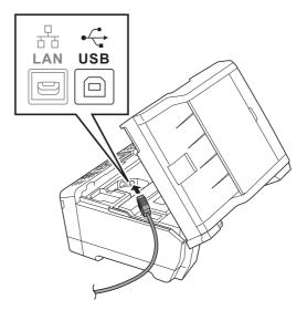
Carefully guide the USB cable into the cable channel and out the back of the machine.
