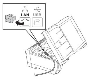
C Carefully guide the network cable into the cable channel and out the back of the machine. Connect the cable to your network.
