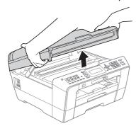
Store the orange protective part in the holder inside the machine as shown.
