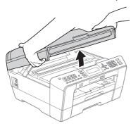
b You will find the LAN socket marked with a symbol inside the machine on the left as shown below. Remove the protective cap and connect the network cable to the LAN socket.
