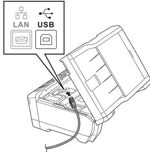
**c** Carefully guide the USB cable into the cable channel and out the back of the machine. Connect the cable to your Macintosh.
