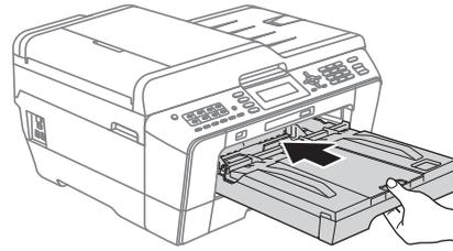
**i** While holding the paper tray in place, pull out the paper support ① until it clicks, and then unfold the paper support flap ②.
