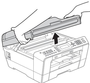
**b** You will find the LAN socket marked with a
