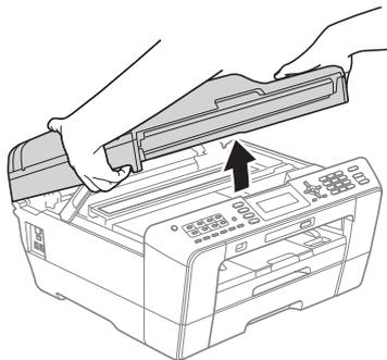
**b** Connect the USB cable to the USB socket marked with a
