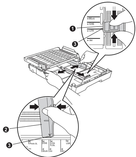
**d** Fan the stack of paper well to avoid paper jams and misfeeds.
