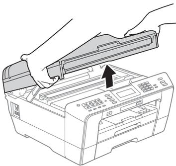
**b** You will find the LAN socket marked with a
