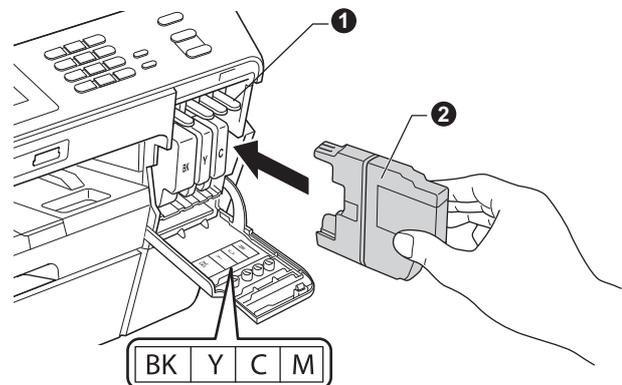
**i** Gently push the back of the ink cartridge marked “PUSH” until it clicks. After all the ink cartridges are installed close the ink cartridge cover.
