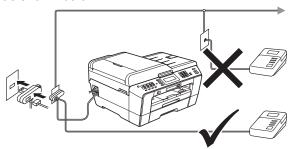
Set the receive mode to External TAD if you have an external answering machine. See Choose a Receive Mode on page 8. For additional details, see Connecting an external TAD (telephone answering device) in chapter 6 of the Basic User's Guide.
