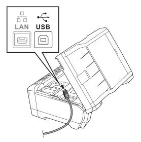
Carefully guide the USB cable into the cable channel and out the back of the machine. Connect the cable to your computer.
