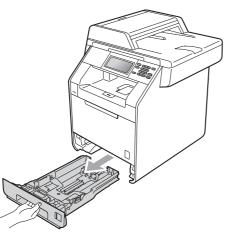
While pressing the green paper-guide release lever (), slide the paper guides to fit the paper size you are loading in the tray. Make sure that the guides are firmly in the slots.
