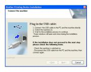
e Connect the USB cable to the USB connector marked with the esymbol on your machine and then connect the cable to your computer.
