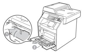
C Press the front cover release button and open the front cover. Remove the silica gel pack 1.
