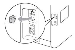
С Connect the network interface cable to the LAN connector and then connect it to a free port on your hub.
