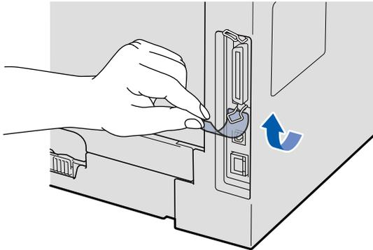
**b** Connect the USB cable to the USB connector on the machine marked with the
