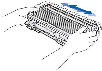
**e** Put the drum unit assembly into the machine until it clicks into place.
