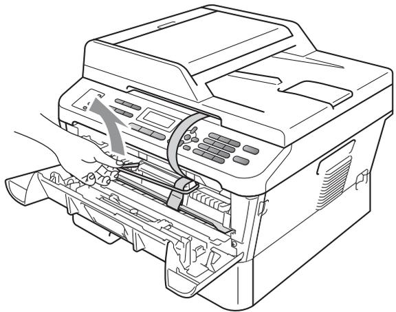
**e** Pull the paper strip to remove the protective material as shown in the illustration.
