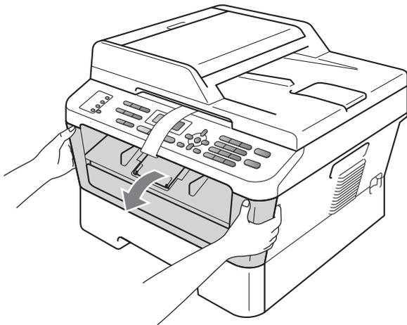
**c** Remove the Silica Pack from the inside of the machine.
