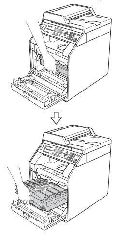
4 Turn the green lock lever (1) at the left of the machine counterclockwise to the release position. Holding the green handles of the drum unit, lift the front of the drum unit and remove it from the machine.
