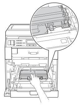
9 Put the belt unit back into the machine. Make sure the belt unit is level and fits firmly into place.
