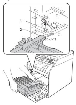
$\mathbf{10}$ Turn the green lock lever (1) clockwise to the lock position.
