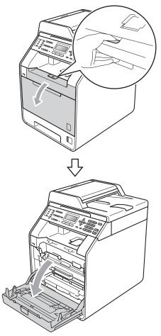
3 Hold the green handle of the drum unit. Pull the drum unit out until it stops.
