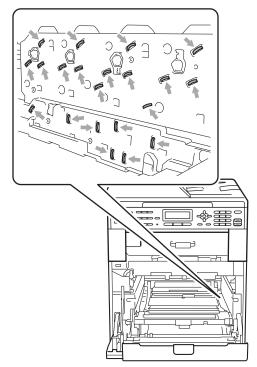
• Hold the green handles of the drum unit when you carry it. DO NOT hold the side of the drum unit.
