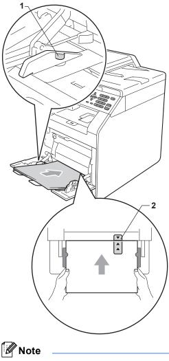
When you are using glossy paper, put only one sheet at a time in the MP tray to avoid a paper jam. 4 Lift up the support flap to prevent paper from sliding off the face down output tray, or remove each page as soon as it comes out of the machine.
