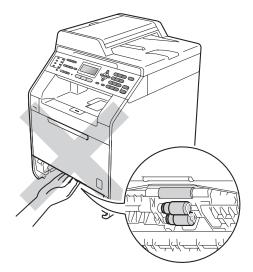
If paper is not caught inside the machine, turn the paper tray over and check underneath the paper tray.
