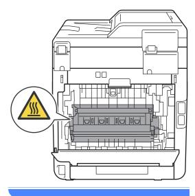
5 Push down and pull the green tabs at the left and right hand sides toward you and fold down the fuser cover (1).
