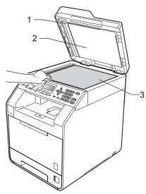
4 In the ADF unit, clean the white bar (1) and the scanner glass strip (2) underneath it with a soft lint-free cloth moistened with water.
