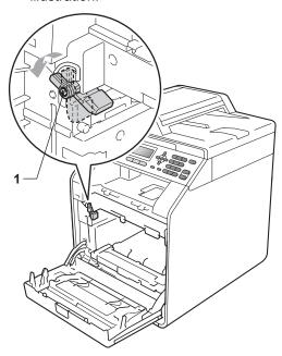
7 Match the guide ends (2) of the drum unit to the ▶ marks (1) on both sides of the machine, then gently slide the drum unit into the machine until it stops at the green lock lever.
