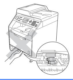
If paper is not caught inside the machine, turn the paper tray over and check underneath the paper tray.
