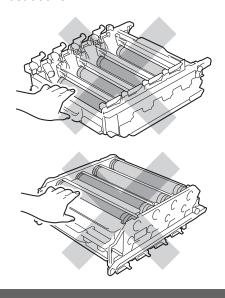
5 Hold the green handle of the belt unit with both hands and lift the belt unit up, then pull it out.
