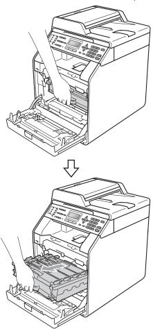
4 Turn the green lock lever (1) at the left of the machine anticlockwise to the release position. Holding the green handles of the drum unit, lift the front of the drum unit and remove it from the machine.
