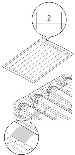
Turn the drum unit gear toward you by hand while looking at the surface of the suspected area.
