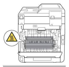
5 Push down and pull the green tabs at the left and right hand sides toward you and fold down the fuser cover (1).
