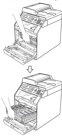
4 Hold the handle of the toner cartridge and slightly push it toward the machine to unlock it. Then pull it out of the drum unit. Repeat this for all the toner cartridges.
