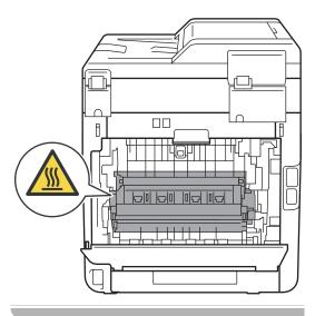
3 Pull the green tabs (2) at the left and right hand sides toward you and fold down the fuser cover (1).
