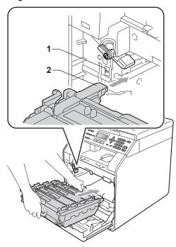
10 Turn the green lock lever (1) clockwise to the lock position.
