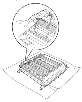
When you have found the mark on the drum that matches the drum dot check sheet, wipe the surface of the drum gently with a cotton swab until the mark on the surface comes off.
