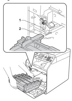
12 Turn the green lock lever (1) clockwise to the lock position.
