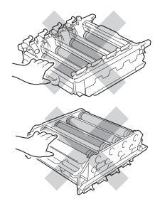
Unpack the drum unit just before you put it in the machine. Exposure to direct sunlight or room light may damage the drum unit. 7 Hold the handle of the toner cartridge and slide the toner cartridge into the new drum unit, then slightly pull it toward you until you hear it click into place. Make sure that you match the toner cartridge colour to the same colour label on the drum unit. Repeat this for all the toner cartridges.
