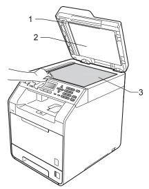
4 In the ADF unit, clean the white bar (1) and the scanner glass strip (2) underneath it with a soft lint-free cloth moistened with water.
