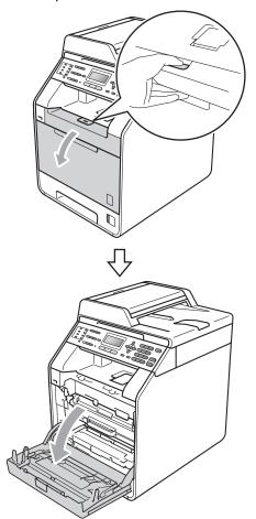
3 Hold the green handle of the drum unit. Pull the drum unit out until it stops.
