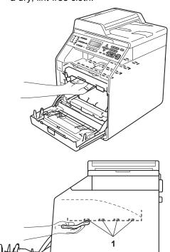
6 Make sure the green lock lever (1) is in the release position as shown in the illustration.
