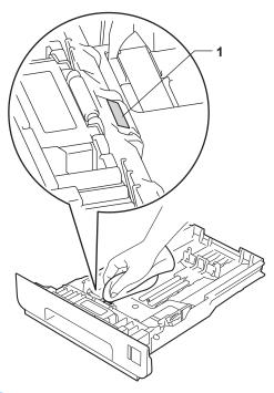
Wipe the two pick-up rollers (1) inside the machine to remove dust.
