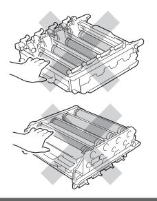
b Hold the green handle of the belt unit with both hands and lift the belt unit up, then pull it out.
