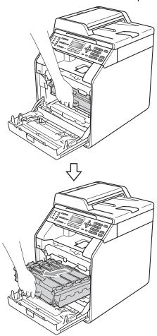
5 Turn the green lock lever (1) at the left of the machine anticlockwise to the release position. Holding the green handles of the drum unit, lift the front of the drum unit and remove it from the machine.
