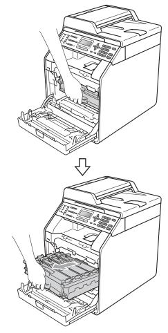
4 Turn the green lock lever (1) at the left of the machine anticlockwise to the release position. Holding the green handles of the drum unit, lift the front of the drum unit and remove it from the machine.
