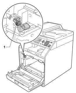
12 Match the guide ends (2) of the drum unit to the ► marks (1) on both sides of the machine, then gently slide the drum unit into the machine until it stops at the green lock lever.
