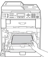
1 Make sure the green lock lever (1) is in the release position as shown in the illustration.
