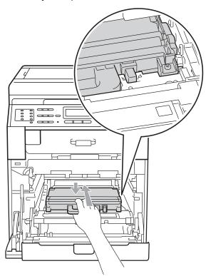
9 Put the belt unit back into the machine. Make sure the belt unit is level and fits firmly into place.
