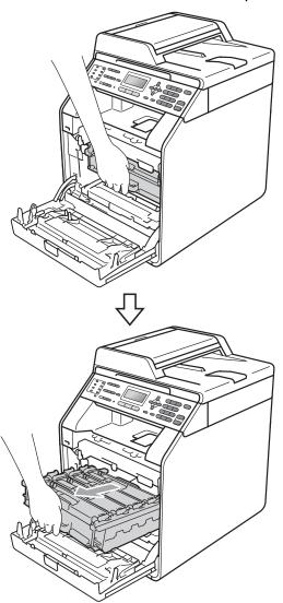
Turn the green lock lever (1) at the left of the machine anticlockwise to the release position. Holding the green handles of the drum unit, lift the front of the drum unit and remove it from the machine.
