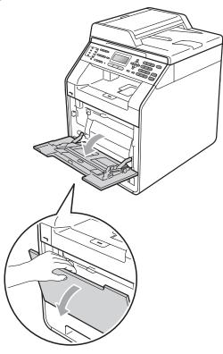
2 Pull out the MP tray support and unfold the flap (1).
