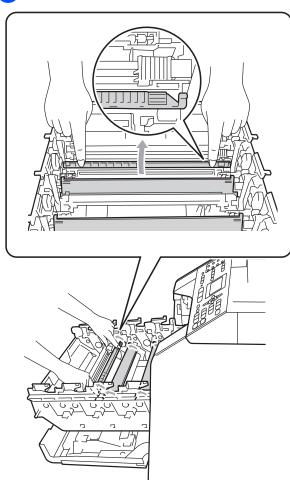
Repeat steps 4 to 6 to clean each of three remaining corona wires. 8 Hold the handle of the toner cartridge and slide the toner cartridge into the drum unit, then slightly pull it toward you until you hear it click into place. Make sure that you match the toner cartridge color to the same color label on the drum unit. Repeat this for all the toner cartridges.
