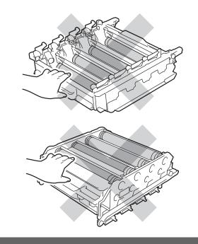
Hold the green handle of the belt unit with both hands and lift the belt unit up, then pull it out.
