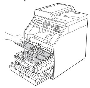
4 Push to release the latches of the corona wire cover (1), and then open the cover.
