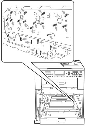
Hold the green handles of the drum unit when you carry it. DO NOT hold the side of the drum unit.  To avoid print quality problems, DO NOT touch the shaded parts shown in the illustrations.
