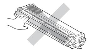
11 Hold the handle of the toner cartridge and slide the toner cartridge into the drum unit, then slightly pull it toward you until you hear it click into place. Make sure that you match the toner cartridge color to the same color label on the drum unit. Repeat this for all the toner cartridges.
