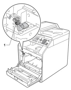
Match the guide ends (2) of the drum unit to the ► marks (1) on both sides of the machine, then gently slide the drum unit into the machine until it stops at the green lock lever.
