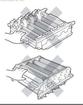
Hold the green handle of the belt unit with both hands and lift the belt unit up, then pull it out.
