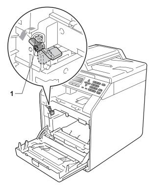
11 Match the guide ends (2) of the drum unit to the ▶ marks (1) on both sides of the machine, then gently slide the drum unit into the machine until it stops at the green lock lever.
