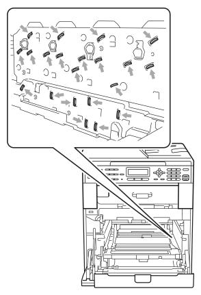
Hold the green handles of the drum unit when you carry it. DO NOT hold the side of the drum unit. 6 Pull out the jammed paper slowly.
