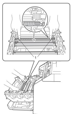
6 Clean the corona wire inside the drum unit by gently sliding the green tab from left to right and right to left several times.
