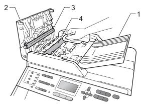
3 Lift the document cover (1). Clean the white plastic surface (2) and scanner glass (3) underneath it with a soft lint-free cloth moistened with water.
