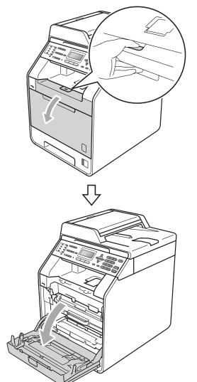
Hold the green handle of the drum unit. Pull the drum unit out until it stops.
