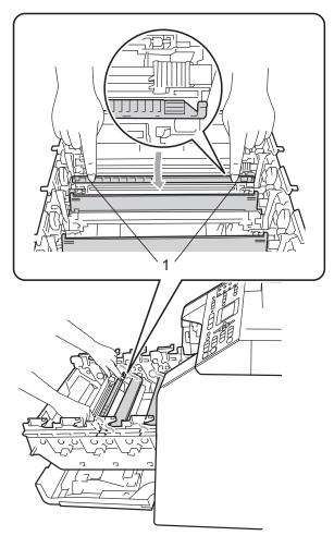
Clean the corona wire inside the drum unit by gently sliding the green tab from left to right and right to left several times.
