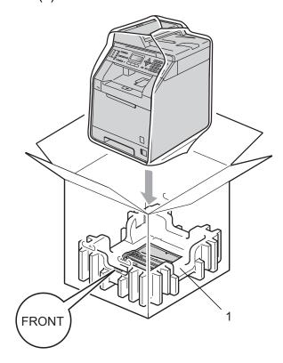
Put the two styrofoam pieces (1) into the carton matching the right of the machine to the "RIGHT" mark on one of the styrofoam pieces, and the left of the machine to the "LEFT" mark on the other styrofoam piece. Put the AC power cord and printed materials in the original carton as shown in the illustration.
