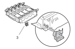
Put a piece of paper (A4 or Letter) on the belt unit to prevent damage to the belt unit.
