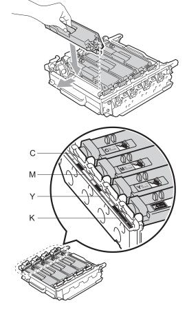
C - Cyan M - Magenta Y - Yellow K - Black 8 Make sure the green lock lever (1) is in the release position as shown in the illustration.
