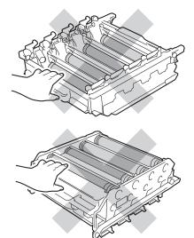
Unpack the drum unit just before you put it in the machine. Exposure to direct sunlight or room light may damage the drum unit. 7 Hold the handle of the toner cartridge and slide the toner cartridge into the new unit, then slightly pull it toward you until you hear it click into place. Make sure that you match the toner cartridge colour to the same colour label on the drum unit. Repeat this for all the toner cartridges.
