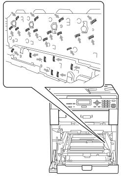
Hold the green handles of the drum unit when you carry it. DO NOT hold the side of the drum unit. Wipe the four scanner windows (1) with a dry, lint-free cloth.
