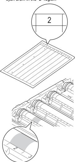
10 Turn the drum unit gear toward you by hand while looking at the surface of the suspected area.
