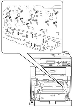
Hold the green handles of the drum unit when you carry it. DO NOT hold the side of the drum unit. 6 Hold the handle of the toner cartridge and slightly push it to unlock it. Then pull it out of the drum unit. Repeat this for all the toner cartridges.
