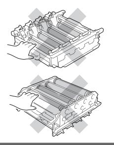
6 Hold the green handle of the belt unit with both hands and lift the belt unit up, then pull it out.
