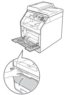
2 Pull out the MP tray support and unfold the flap (1).
