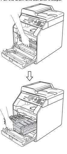
Turn the green lock lever (1) at the left of the machine anticlockwise to the release position. Holding the green handles of the drum unit, lift the front of the drum unit and remove it from the machine.
