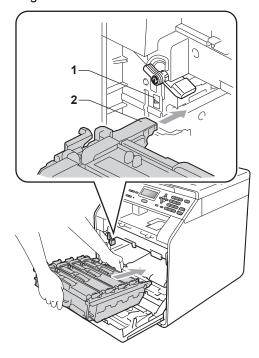
10 Turn the green lock lever (1) clockwise to the lock position.
