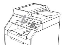
You can still use the machine while the scanner is up. To close the scanner, push it down with both hands.
