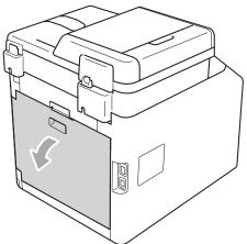
6 Pull down the two grey levers, one on the left-hand side and one on the righthand side, to the envelope position as shown in the illustration below.
