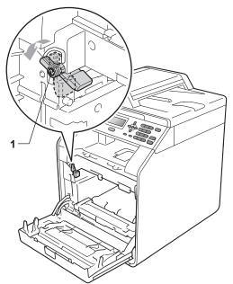
14 Match the guide ends (2) of the drum unit to the ► marks (1) on both sides of the machine, then gently slide the drum unit into the machine until it stops at the green lock lever.
