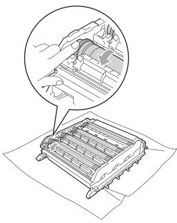
11 When you have found the mark on the drum that matches the drum dot check sheet, wipe the surface of the drum gently with a cotton swab until the dust or paper powder on the surface comes off.
