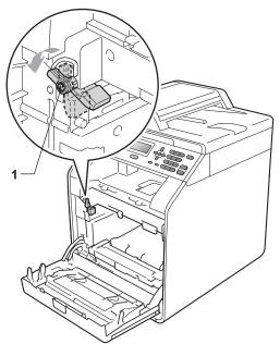
1 Match the guide ends (2) of the drum unit to the ► marks (1) on both sides of the machine, then gently slide the drum unit into the machine until it stops at the green lock lever.
