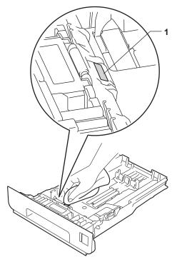
4 Wipe the two pick-up rollers (1) inside the machine to remove dust.
