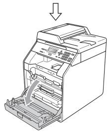
2 Hold the green handle of the drum unit. Pull the drum unit out until it stops.
