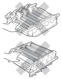
• Unpack the drum unit just before you put it in the machine. Exposure to direct sunlight or room light may damage the drum unit.
