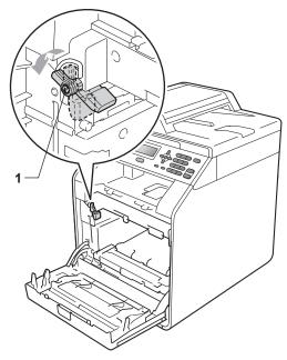
7 Match the guide ends (2) of the drum unit to the ▶ marks (1) on both sides of the machine, then gently slide the drum unit into the machine until it stops at the green lock lever.
