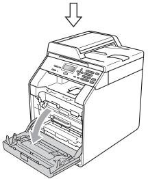
3 Hold the green handle of the drum unit. Pull the drum unit out until it stops.
