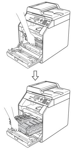
3 Hold the handle of the toner cartridge and slightly push it toward the machine to unlock it. Then pull it out of the drum unit. Repeat this for all the toner cartridges.
