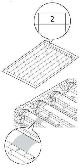
10 Turn the drum unit gear toward you by hand while looking at the surface of the suspected area.
