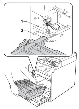
**15** Turn the green lock lever (1) clockwise to the lock position.
