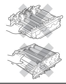
5 Hold the green handle of the belt unit with both hands and lift the belt unit up, then pull it out.
