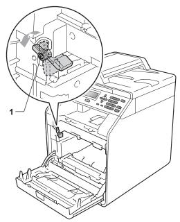
9 Match the guide ends (2) of the drum unit to the ► marks (1) on both sides of the machine, then gently slide the drum unit into the machine until it stops at the green lock lever.
