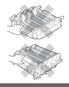
7 Turn the drum unit over by holding the green handles. Make sure that the drum unit gears (1) are on the left hand side.
