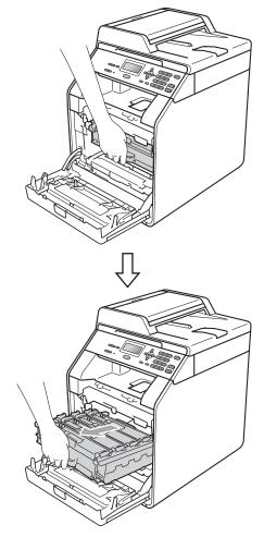
4 Hold the handle of the toner cartridge and slightly push it toward the machine to unlock it. Then pull it out of the drum unit. Repeat this for all the toner cartridges.
