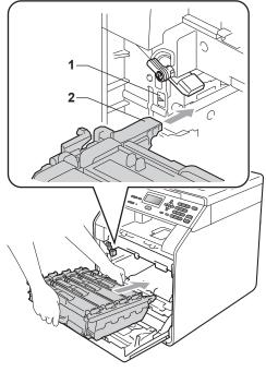
Turn the green lock lever (1) clockwise to the lock position.
