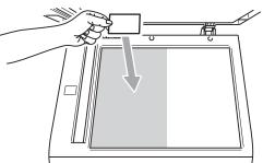
Even if a document is placed in the ADF, the machine scans the data from the scanner glass for 2 in 1 ID copy.
